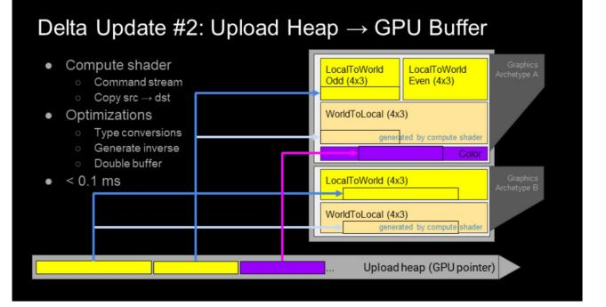
The second step of the data upload process is to go through the linear upload heap data array and scatter the modifications around the large ByteAddressBuffers containing the mirrored ECS state.
