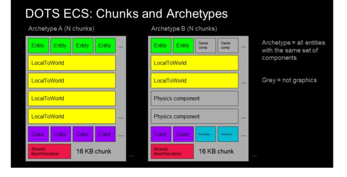
DOTS ECS has a chunk based data model. Entities are split to archetypes based on their component set. Entities with different archetype are split to different chunks. DOTS uses fixed size 16 KB chunks. This makes memory allocation trivial.
